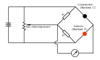
Note: The value R1 is arbitrary, since the function of R1 is to balance the bridge. 1  $k\Omega$  is suggested.
